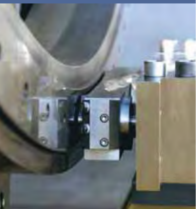
Rotocal Radial rotary union for large shafts with diameters of up to 3 m
