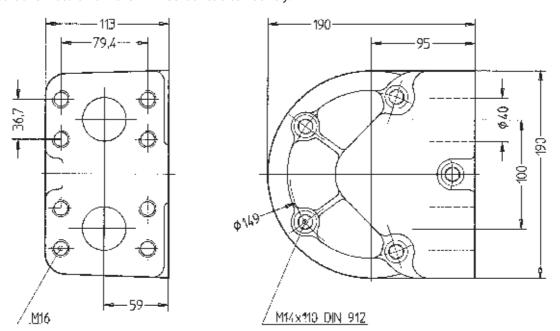
**Distributor J40** connections SAE 2", 6000 psi (420 bar) for all hydraulic motors from the HMT-40.. serie standard.
