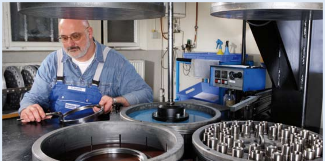
Lapping of sealing surfaces
