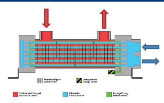
Based on their existing hybrid heat exchangers from the SCM-Series, Universal Hydraulik developed a new high efficiency fail-safe heat exchanger, the SCM/FS. The advantages of the hybrid design, such as a compact size or an internal bypass valve of the newest generation, can be completely utilized.
