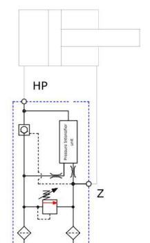
Inlet flow: Min. 2 LPM to max. 20 LPM
