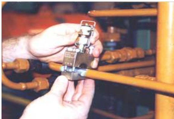
Installation on non-pressurized pipe Serv-Clip 2
