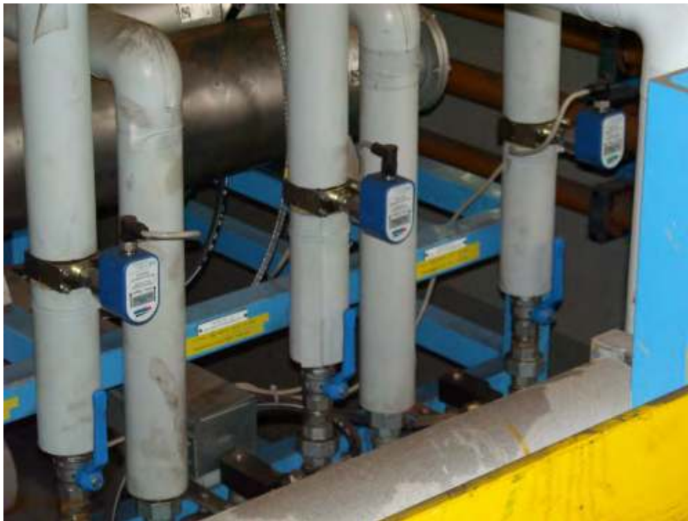
Picture 4: Control of a lubrication oil line with flow rate sensors and Serv-Clip -2 at a continuous pickling line.
