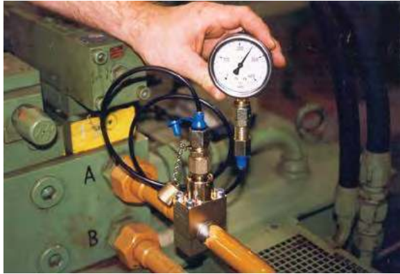
Installation on pressurized pipe Serv-Clip 1
