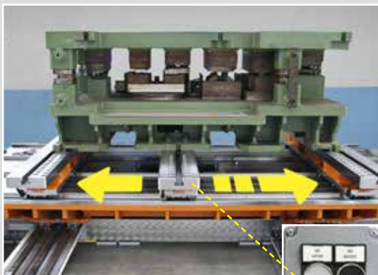
Hydraulic motors in parallel to move the parallel supports by simply pressing a single button to find the right to left position.
