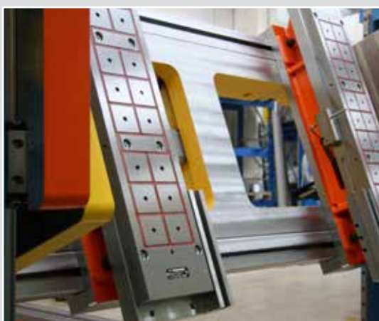
With permanent magnet parts (highly practical for clamping in just a few seconds with just the push of a button).
