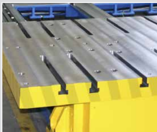
"T" slots on the whole surface.
