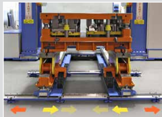
Lower carriages that slide right and left.
